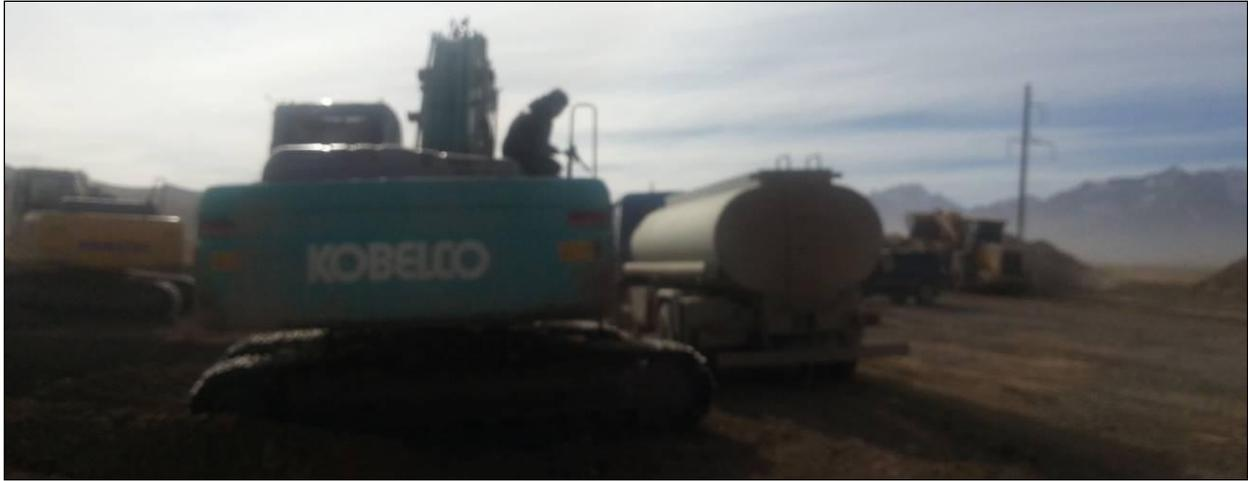
Figure 32: Onsite refueling of plant by dedicated refueling truck
