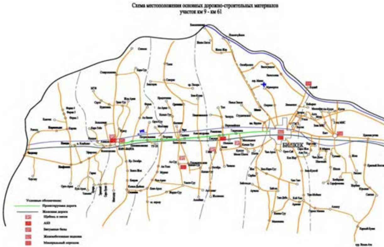
Fig. 6: Borrow areas along the road section Bishkek – Kara Balta
